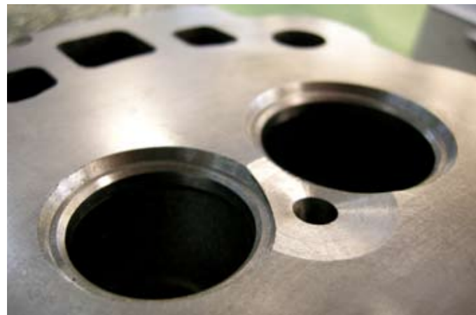
Stainless steel valves increase cylinder head durability.
