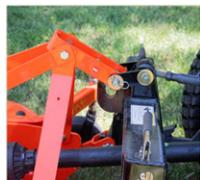
An optional link is available for implements that have a floating top link allowing unit to follow the contour on the ground.
